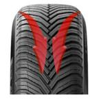
tire's sidewall (Note: these markings only appear on one side of the tire). To maintain their performance and safety advantages, it's crucial to mount them correctly, ensuring that all four tires rotate in the intended direction. When correctly mounted, the arrow points toward the front of the vehicle. Incorrectly mounted directional tires lead to reduced effectiveness, decreasing the tires hydroplaning resistance, handling and traction benefits.
