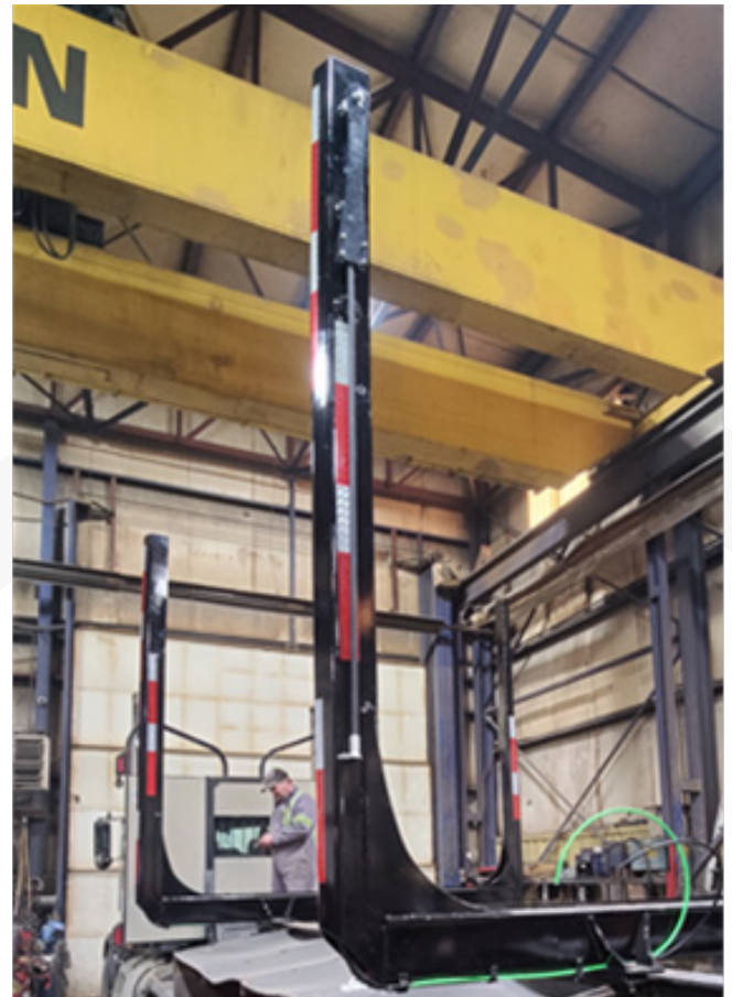
Figure 1. Trinder wrapper thrower (1.8 m arm with hook at the end)
