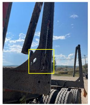
Figure 18. ANR SLM installed 2 ft lower than optimal on the stake creating the possibility of grapple hitting the tires.
