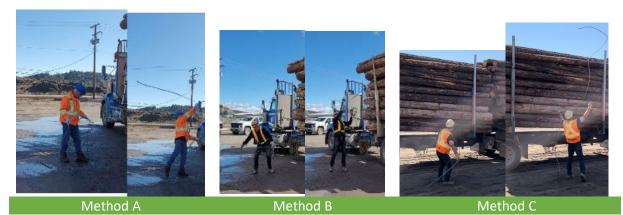
Figure 9. Alternative throwing methods using 5/16" steel wrappers.
