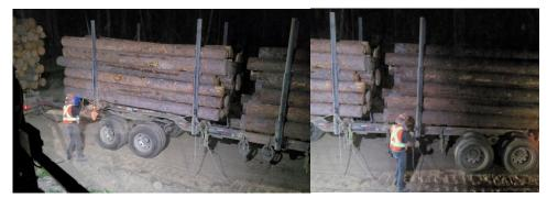
Figure 13. Driver setting up wrappers on the loader-assist tools at nighttime.
