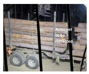
Figure 15. ExTe Long Life arms yet to be retracted to the rested position.
