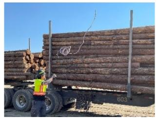
Figure 32. Driver throwing a synthetic wrapper.
