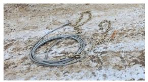
Figure 20. 3/8" steel wrapper.
