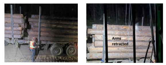
Figure 17. Setting up the wrapper on ANC SLM at nighttime (left) and loader draping the wrapper over the load (right).
