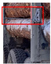
a) ANC spring-loaded mechanism (SLM) Figure 10. Loader assist tools.
