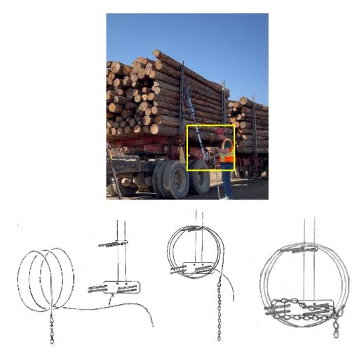
Figure 28. Coiling of wrapper onto RotatorSaver (Source: RotatorSaver, reproduced with permission).
