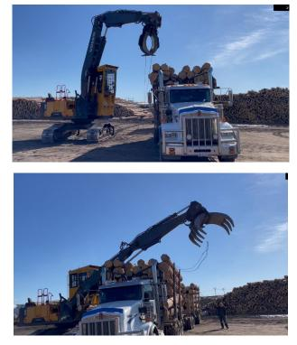
Figure 8. Loader draping the wrappers over the load.
