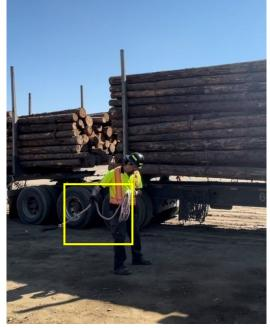
**Synthetic wrapper Synthetic tiedown** Figure 33. Lightweight synthetic wrapper/tiedown used for throwing.
