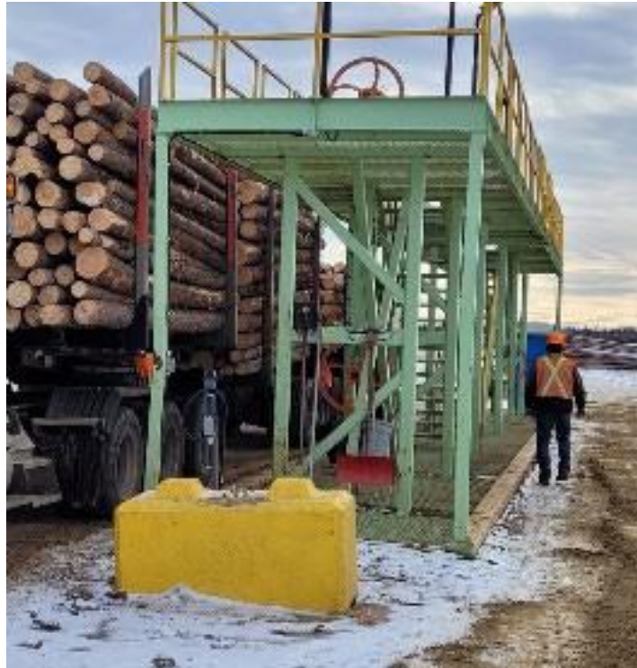
Figure 35. Platform in a reload site for throwing wrappers from an elevated position.
