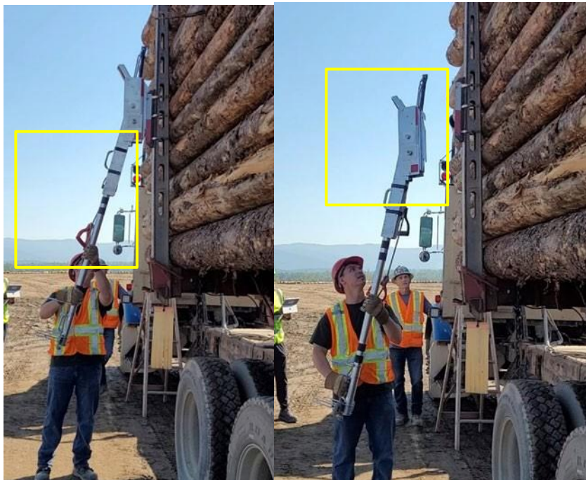
Figure 27. Installing the RotatorSaver onto the bracket mounted on the stake.
