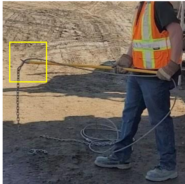
b) Position the pole hook onto the second link from the collar of one of the wrapper ends
