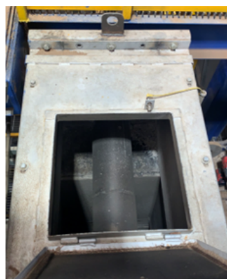
Picture 1 – view into the hatch on day 2 after the furnace burned out
