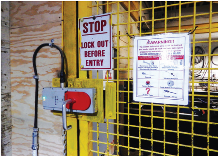
Part of the CSID system, showing magnetically controlled gates tied to operation of the planer.
