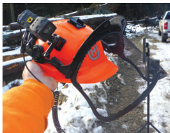
Field testing of fallercams continues prior to a decision being made this spring as to whether they are effective tools for evidence gathering for supervisor certifications and training.
