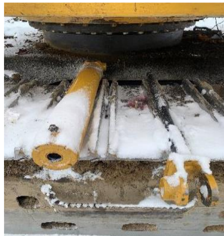
Replaced cab tilt cylinder failure
