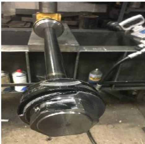
Initial cab tilt cylinder failure due to counterbalance valve
