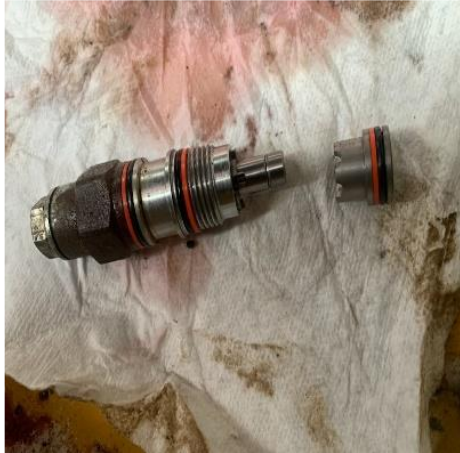
Failed Counterbalance Valve
