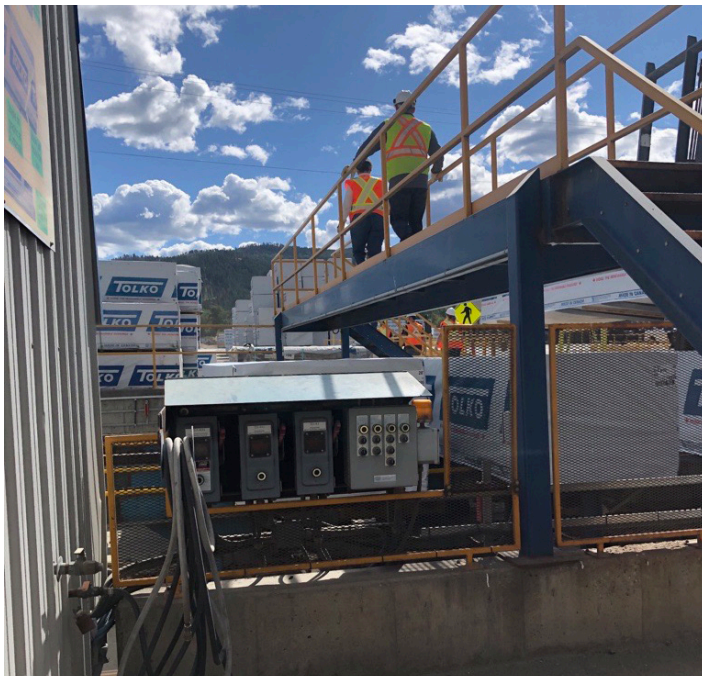
An Inherently Safer Design (ISD – minimization) that removed the hazard of workers walking in front of the package outfeed forklift zone.
