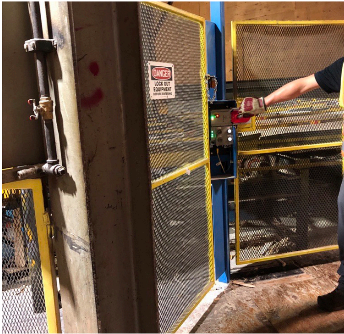
Control System Isolating Device (magnetic lock) on a perimeter gate is at the top of the hierarchy of controls.
