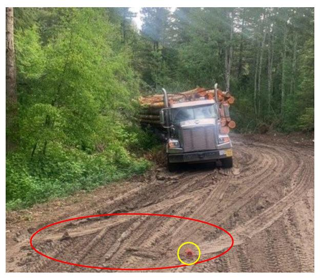
The truck's steering tires travelled forward to the orange tape measure (in yellow circle) then the driver backed up, unfortunately putting him closer to the edge. The tracks show the forward progress of the truck before it ran out of room to manoeuvre.
