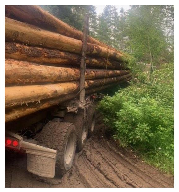
Rear view at the cut corner shows that if workers attempted to pull the truck forward the trailer would clearly leave the road. It's important to recognize an upset condition and be ready to seek assistance.
