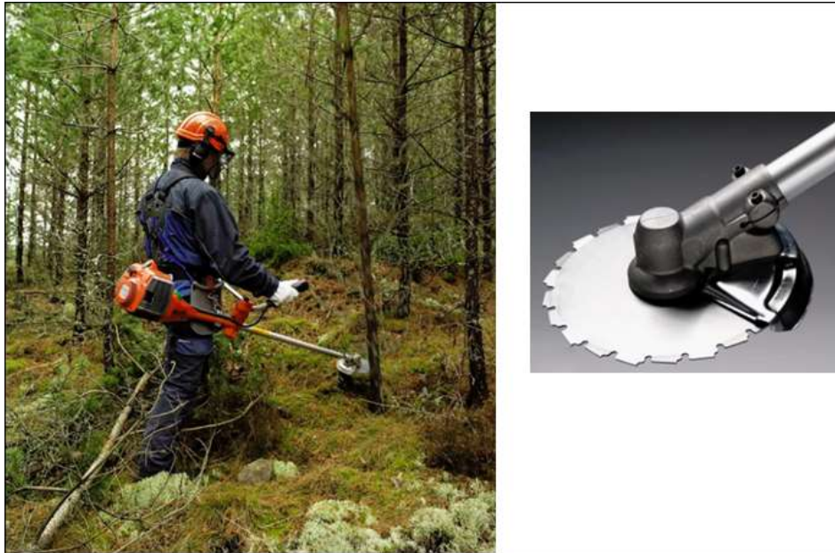
Brush saw (images from Husqvarna https://www.husqvarna.com/us/products/clearing-saws )
