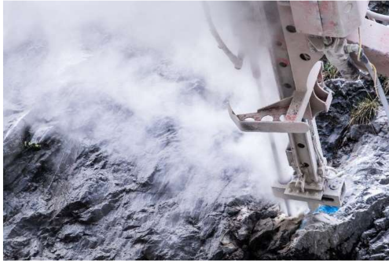
Rock drill creating dust containing silica
