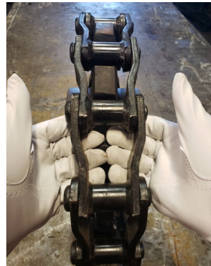
Incorrect Hand Placement
