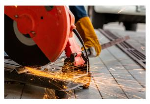
and walk behind models. Abrasive saws use composite friction disk blades to abrasively cut through the material.
