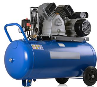
compressed air, then, is held in the tank until used. The energy contained in the compressed air can have different uses, commonly for air powered tools. When the air is released, the tank depressurizes. When tank pressure reaches its lower limit, the air compressor turns on again and re-pressurizes the tank.
