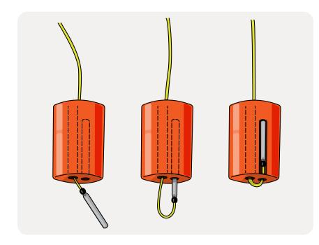
A detonator is threaded through a tunnel in a cast booster (left) and then inserted into a detonator well (centre and right).
