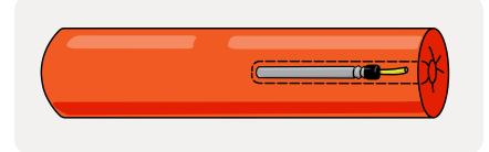
A deteriorated detonator is embedded in a stick of dynamite in preparation for destruction by detonation.
