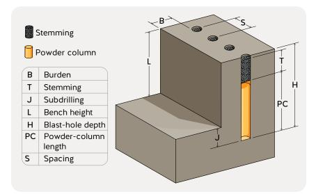
The top and side view of a bench with an even free face. Some key factors in blast pattern design are labelled.
