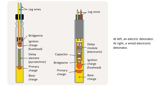
In a wired electronic detonator, the wires are connected to a circuit board. This provides a level of separation where safety features are incorporated.
