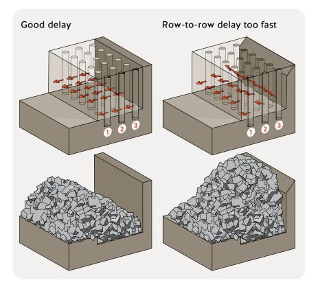
Piling and uplift resulting from different delay timings
