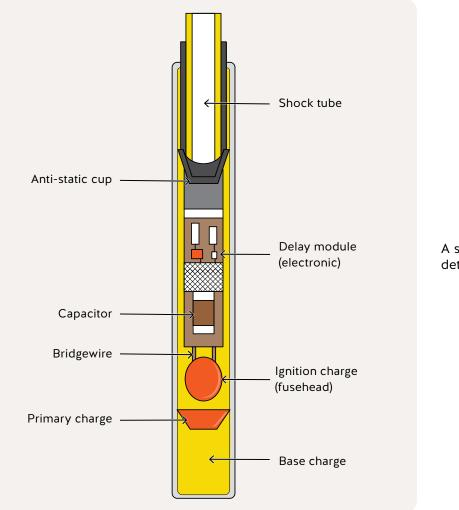
A shock tube-based electronic detonator
