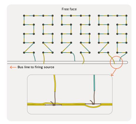
The main drawing shows a multiple series circuit made up of three series with 20 holes per series. The inset shows how one series is tied into the bus line using duplex wire.
