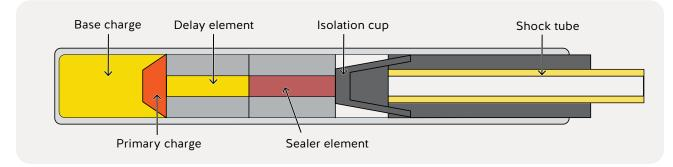
Cutaway view of a shock tube detonator
