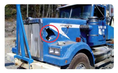
Fly rock thrown from a poorly controlled blast damages a vehicle.
