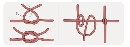
At left, a square or reef knot. At right, a double half hitch.
