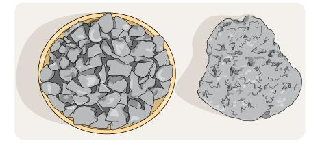
Stemming material immediately above a charge before a blast (left) and after (right). The blast compacts the stemming material into a solid plug.
