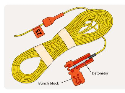
A surface-delay assembly with the detonator end contained in a removable bunch block
