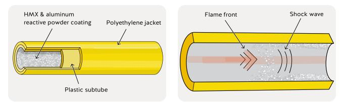
At left, a cutaway view of shock tube. At right, a cutaway view of the reactive powder igniting and generating a shock wave inside a shock tube.
