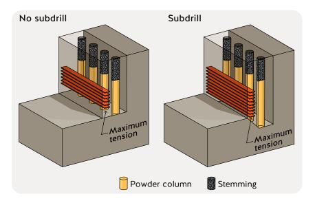
Proper subdrilling can extend the maximum tension zone down to include the bottom of the face. This helps to achieve the desired grade. Too much subdrilling increases ground vibration. Too little subdrilling can lead to high bottom and boulders (oversize material) that may require additional blasting. No subgrade drilling is required if there is rock with horizontal bedding at the desired grade.
