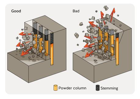
The results of adequate confinement of explosive gases (left) and inadequate confinement (right). The collar length (i.e., the amount of stemming) and the size of the stemming materials work together to confine the explosive gases and control air blast, fly rock, and backbreak.
