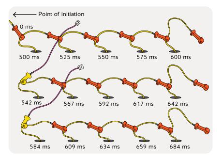
This is an example of calculating timing, including downhole delays and surface delays. The delay times are marked.
