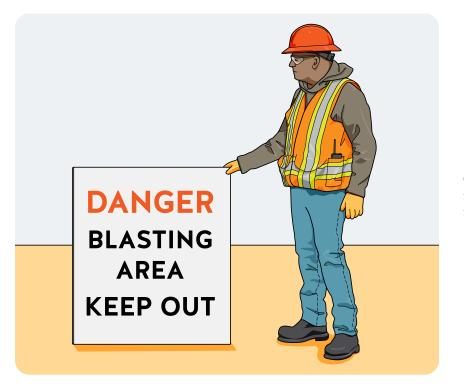
Guards must be posted in safe locations. Signs cannot substitute for guards.
