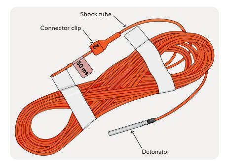
A single-delay assembly with a connector clip
