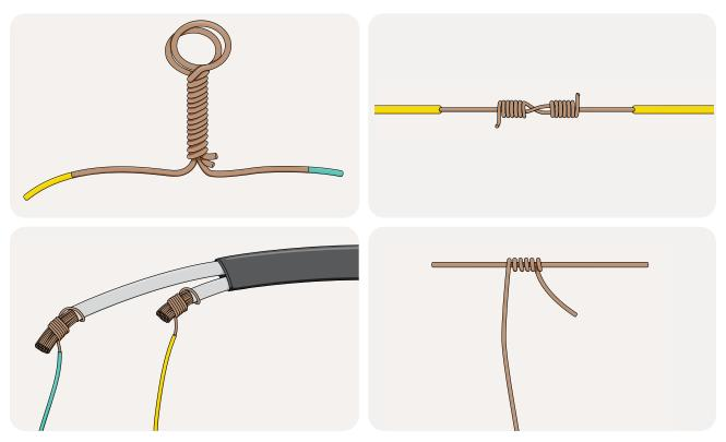
Clockwise from top left: loop-twist connection, western union connection, straight wrap connection, and blasting circuit connected to firing cable
