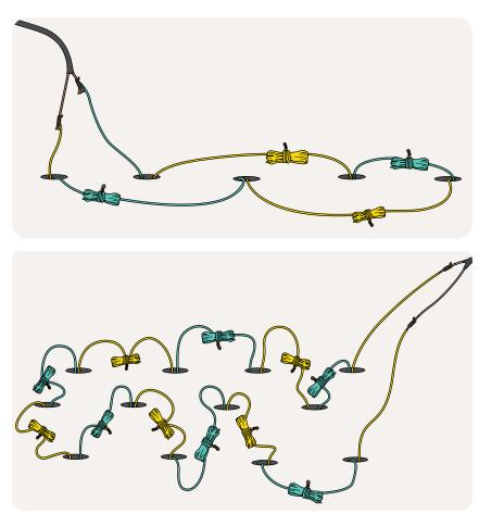
At top, a single series circuit set up in a single row. Loop-twist knots are used to connect one detonator's leg wire to the next detonator's leg wire.
