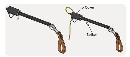
At left, a hand starter. At right, an armed hand starter, shown just before releasing the striker.
