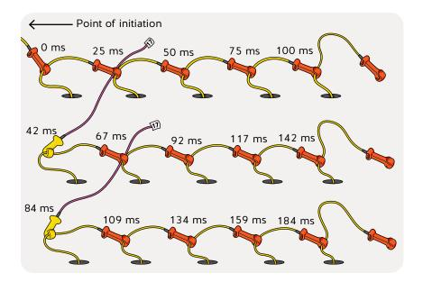
This is an example of using surface delays to fire additional rows of dual-delay assemblies. The surface delay times are marked.
