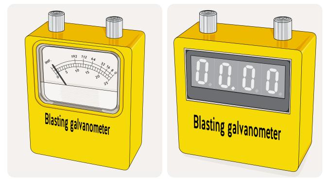
Examples of blasting galvanometers, in analog (left) and digital (right) models
