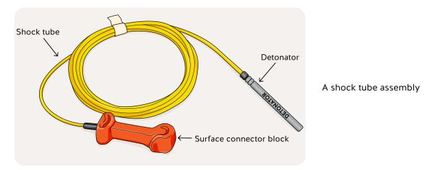
A shock tube assembly is a non-electric type of initiation system. Shock tube assemblies are widely used and are highly preferred in industry over electric initiation. That's because of their electrical insensitivity, durability, flexibility, and ease of *hookup*. The main advantage of a shock tube assembly is its lower sensitivity to stray current. The main shortcoming is the inability to test the circuit prior to initiation.
