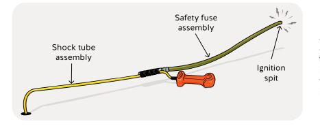
An example of a safety fuse assembly initiating a shock tube assembly and showing ignition spit. (This application would only be acceptable in a remote operation.)
