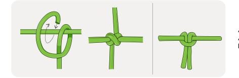
At left, a clove hitch. At right, a double wrap half hitch.
