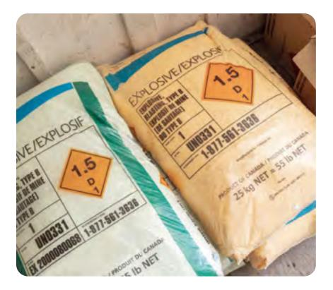
Blasting agents are either dry (free-running) or slurry products. Most dry types of ANFO mixtures have no water resistance, so a plastic *liner* (sock) may be required for wet holes. Dry products are generally supplied in bulk or packaged in bags with oil- and water-resistant liners. When free-pouring ANFO, follow the manufacturer's recommendations for the minimum diameter of the drill hole. These will vary between suppliers.
