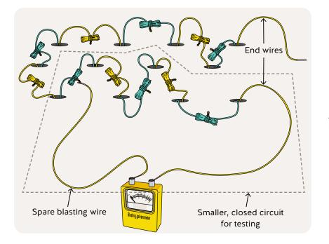
An example of the process for locating a break in a circuit
