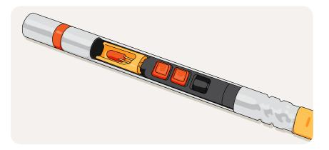
An electronic detonator with part of the shell removed to reveal the internal design
