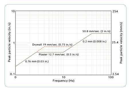
In the Z-curve, allowable levels of vibration frequency and intensity fall below the lines shown. Vibration levels that are higher than the limits appear above the lines. (Source: Report of Investigations 8507, USBM)
