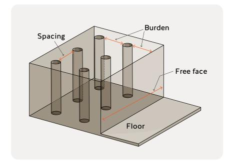
The burden and the spacing give the blaster the initial pattern for blast-hole layout and drilling.
