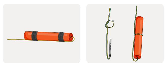
Ensure that the detonator is securely fastened to the cartridge by doing one of the following:
