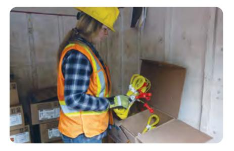
A worker holds several standard 25/500 ms dual-delay shock tube assemblies.
