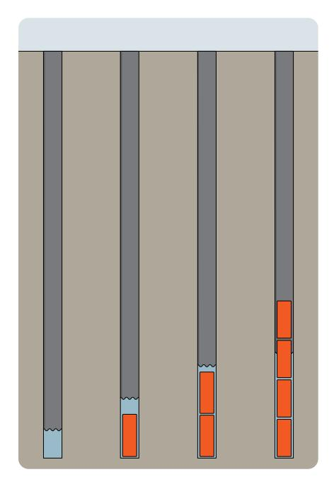
In some cases, such as in solid rock, blasters can use cartridges to displace low levels of water in a blast hole.
