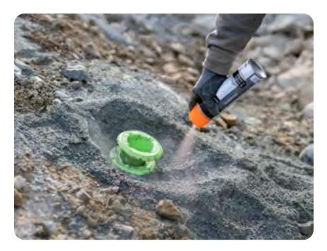
Marking an anomalous hole with double cones and spray paint The driller can be of great help in assessing rock variations that are not apparent from the surface. The driller should watch for the following signs and communicate them to the blaster:
