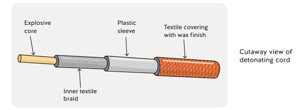
There are several types of detonating cord. The strength of the explosive core load can vary between types, as can the quality of the outer covering and its flexibility. Thinner, more flexible detonating cords can be tied together and used in a wide variety of applications.
