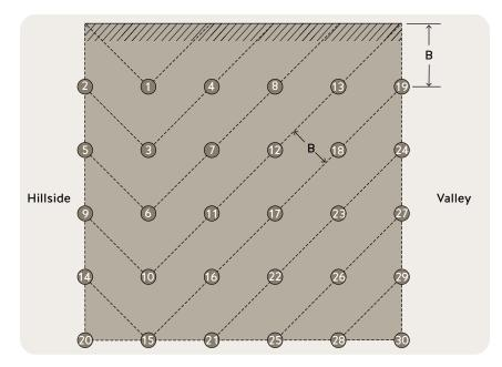
On steep hillsides, the outer row of holes has very little depth. The depth-to-burden ratio (stiffness ratio) should never be less than 1. Large-diameter holes can be used where more depth is available (i.e., higher up the slope). However, the blast hole diameter, spacings, and burdens should be reduced on the lower edges of the slope. This involves changing the drill steel and bit to a smaller size.
