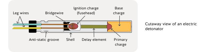
Pressed into the base end of the shell is a composite charge of heat-sensitive lead azide (the primary charge) and high-explosive PETN (the base charge).
