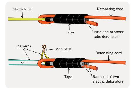
Methods for attaching detonators to detonating cord. The top image shows detonating cord taped to a shock tube detonator. The bottom image shows detonating cord taped to two electric detonators.
