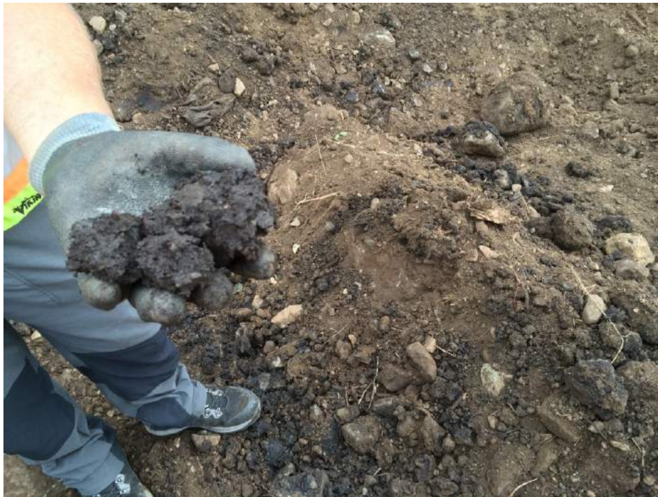
Soil contaminated with used oil (hydrocarbons) at an old forestry shop site on Vancouver Island. Photo credit: Chris Cole, RPF, P. Eng.
