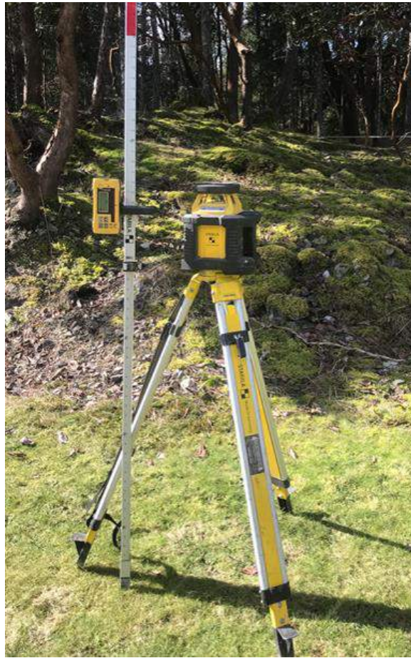
Automatic leveling rotary laser. Image Credit: Chris Cole, RPF, P. Eng.
