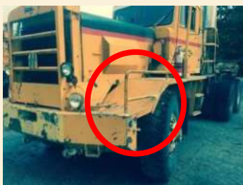
After: handrail installation allows for workable 3-point contact.
