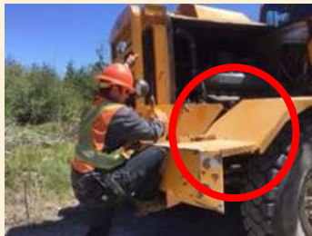
Before: impossible for worker to execute safe 3-point contact.
