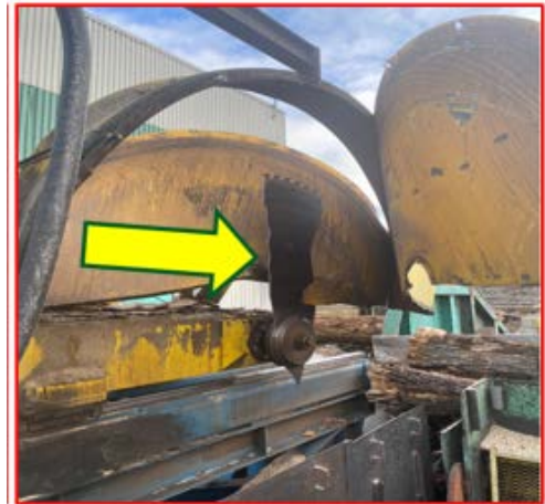
Cut-Off saw blade after breakage
