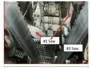
The foreground right saw is a new saw #3, and the saw being removed as #1 (saws to the left are #2 & #4) Filer was also located below the platform to the left.
