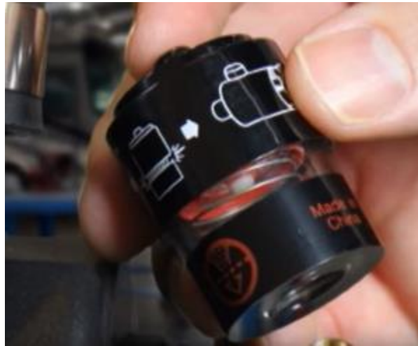
Air intake restriction indicator – photo by Chris Cole, RPF, PEng
