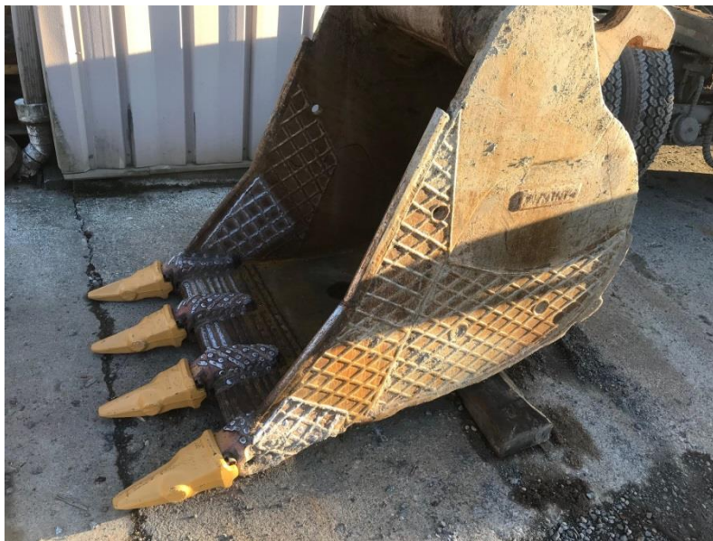
Bucket with teeth recently replaced. Photo by Chris Cole, RPF, P.Eng.
