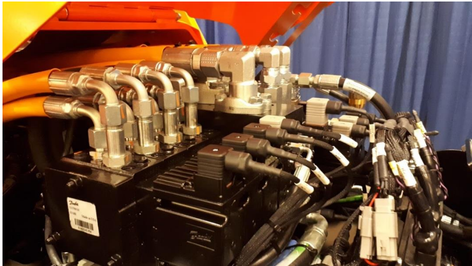
Main lines and labeled pilot lines (inside a log processing attachment)
