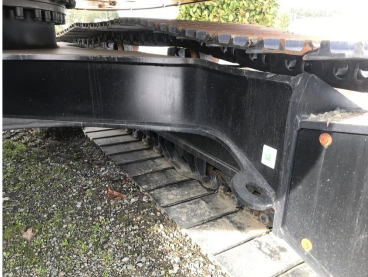
Photo showing inside of track rail and pads. Photo credit: Chris Cole, RPF, PEng
