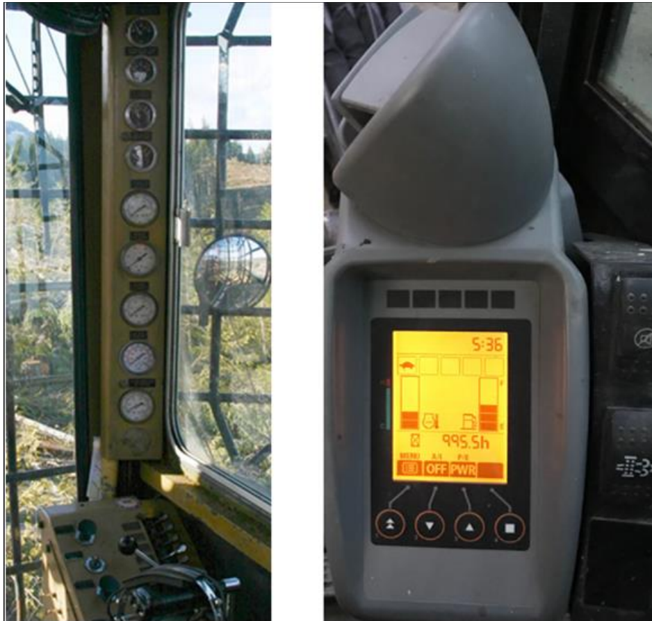
Instrument groups. Needle-and-scale gauges in left photo (from ITA HEO manual) and digital gauges in right photo (from Chris Cole, RPF, PEng)
