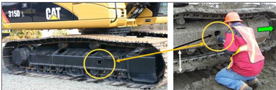
Adjusting track tension (photo from ITA HEO manual)
