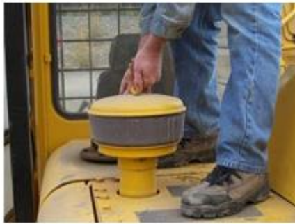
Emptying the dust bowl (photo from ITA HEO manual)
