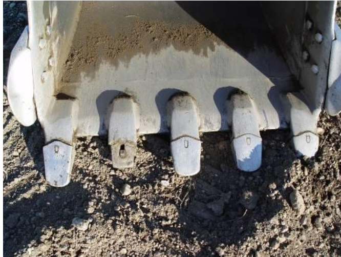
Bucket missing replaceable tooth (photo from ITA HEO manual)
