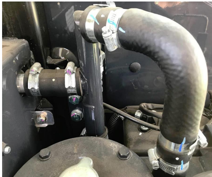
Hose clamps and hydraulic hose fittings marked for tightening (photo from Chris Cole, RPF, PEng)
