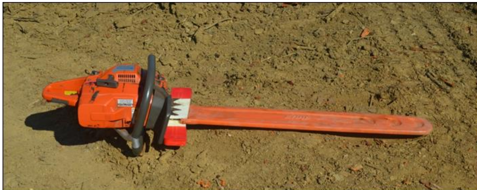
Figure 24: Chain cover and dogs guarded for transport
