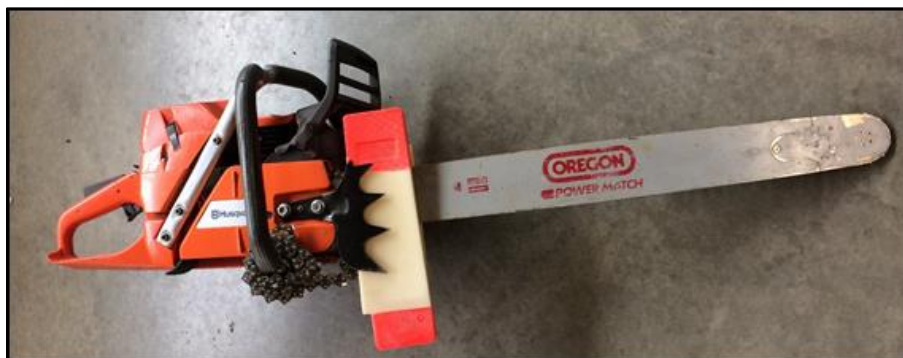
Figure 11: A chainsaw with the dogs guarded
