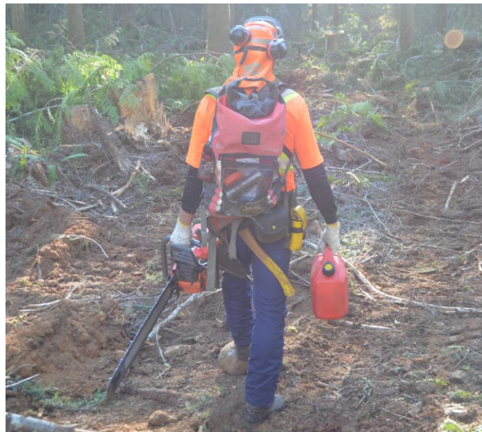
Figure 22: Correct way to carry chainsaw, tools and equipment.
