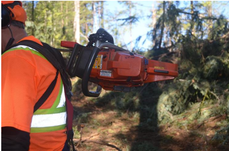
Figure 23: Chain removed and dogs guarded for transport
