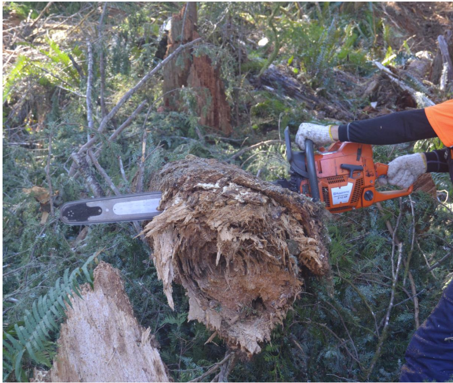
Figure 25: Operating the chainsaw with the right hand.
