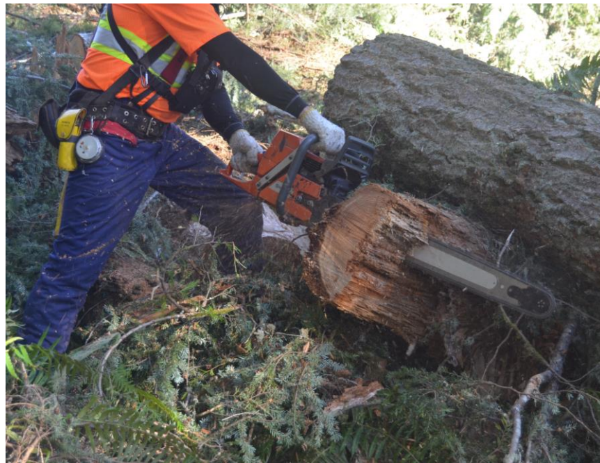
Figure 26: Operating the chainsaw with the left hand.
