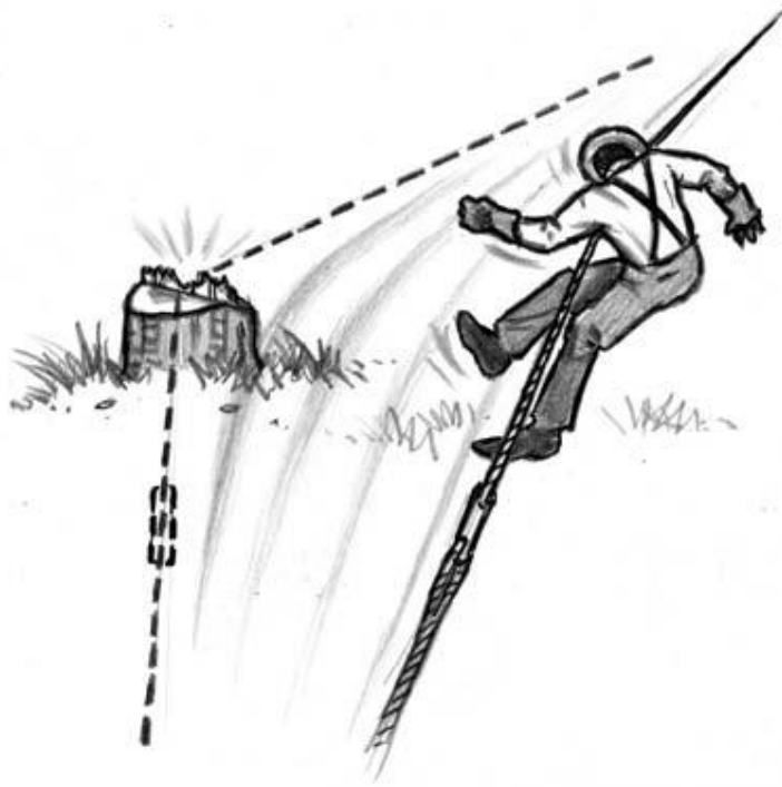
A line caught on a stump can suddenly break free
