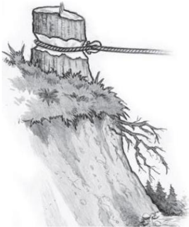
Stump disturbed by grade construction
