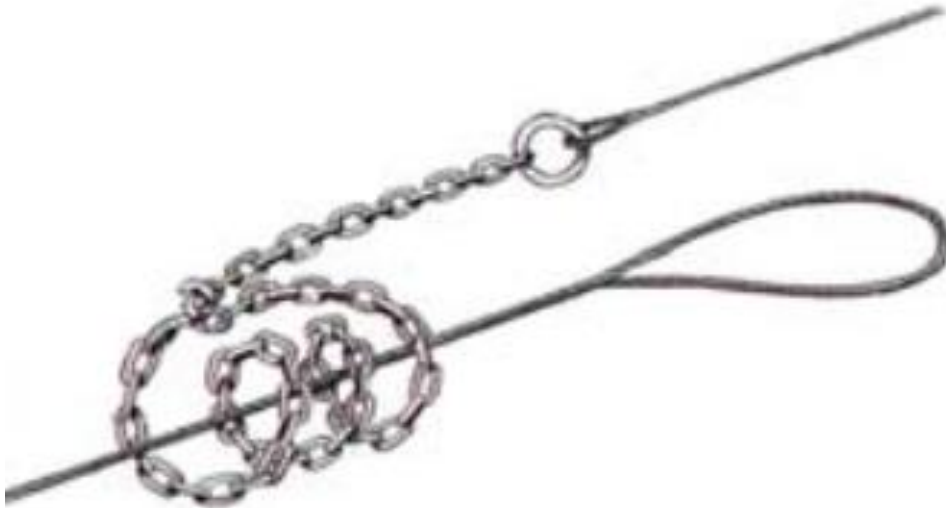
Pass chain wrapped against the pull
