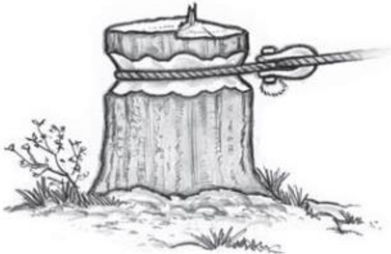
Improper notching: too close to top
