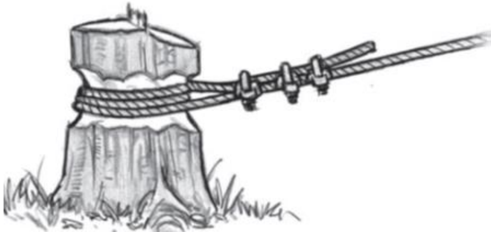
Guyline secured with cable clips
