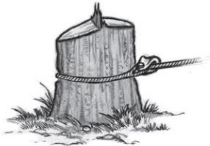
Improper notching: shallow
