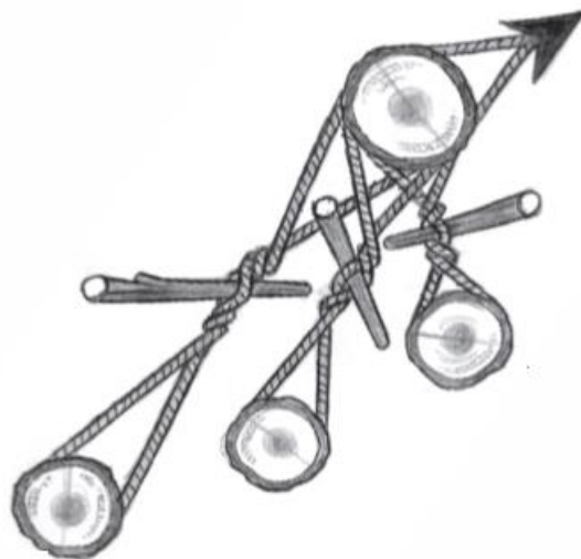
Less effective setup: alignment not in lead
