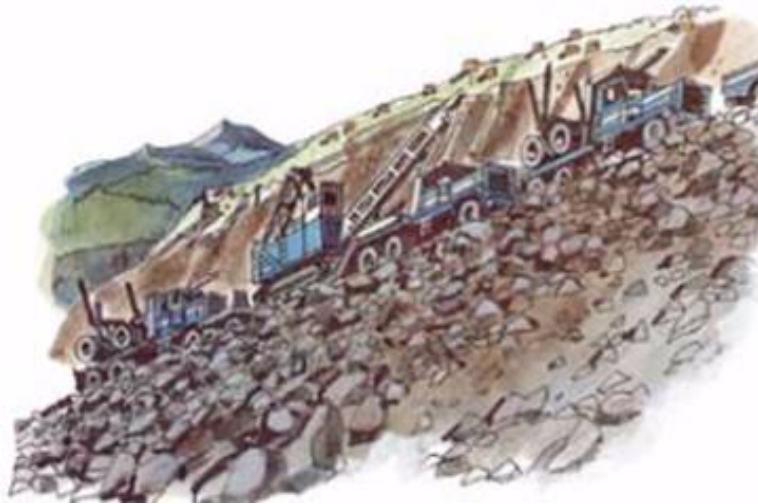
Push and pull trucks assisting lowbed on steeper grade
