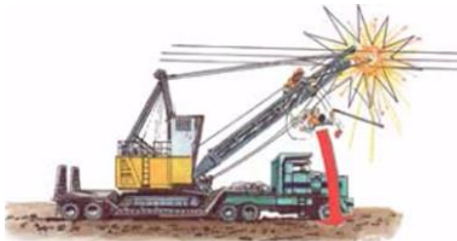
A worker contacting a power line with a lifting stick can be electrocuted. Do not try to clear the line
