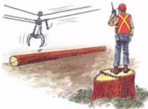
Stand in a safe position when talking a grapple onto a log
