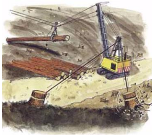
These guylines are out of lead, causing stump pull and machine rocking
