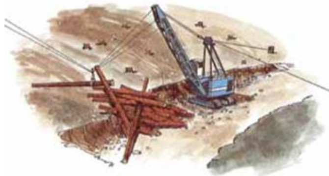
Unstable logs make landing logs hazardous
