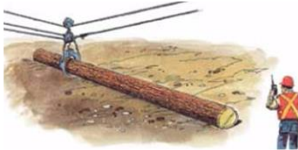
Grapple tightened back on log
