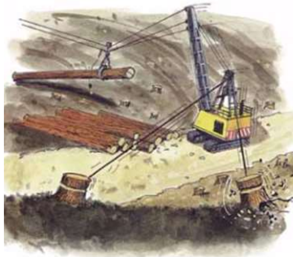
These guylines are out of lead, causing stump pull and machine rocking
