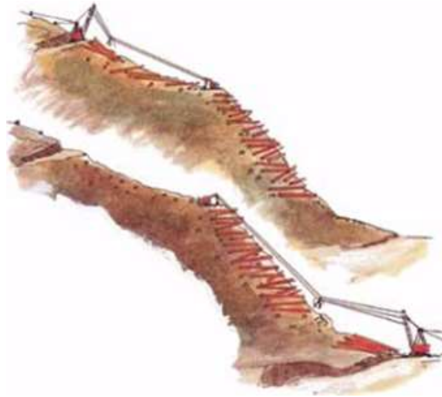
Splitting the logging setting by logging uphill and downhill
