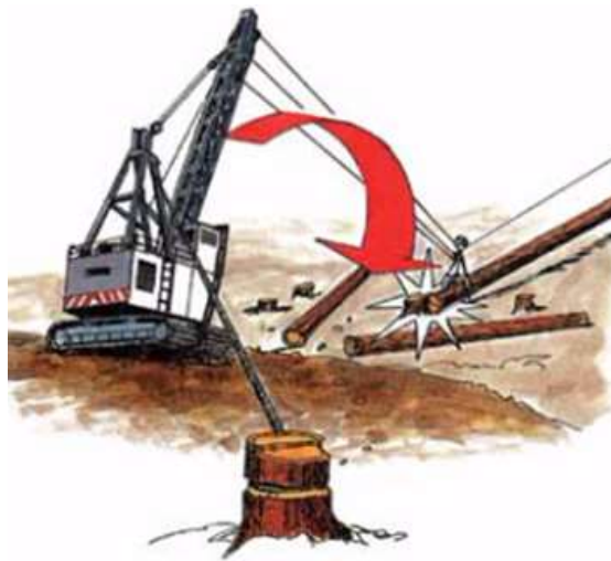
A grapple yarder with a single guyline out of lead can be pulled over
