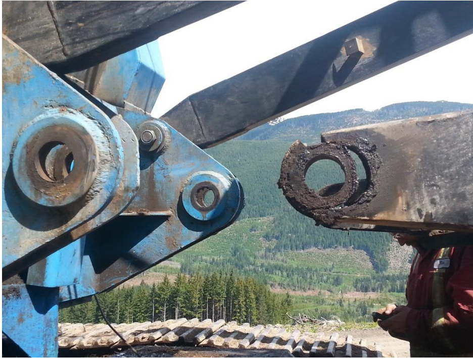
Broken weld not found on inspection
