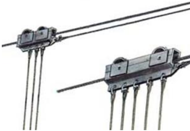
Shotgun carriages with multiple chokers attached
