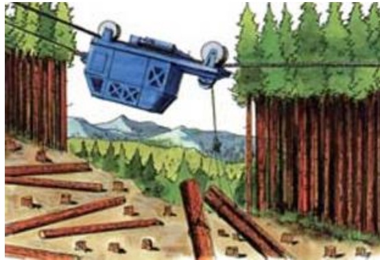
Radio-controlled carriage - no haulback
