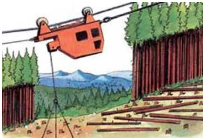
Radio-controlled carriage with haulback attached
