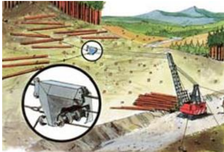
Mechanical slack-pulling carriage
