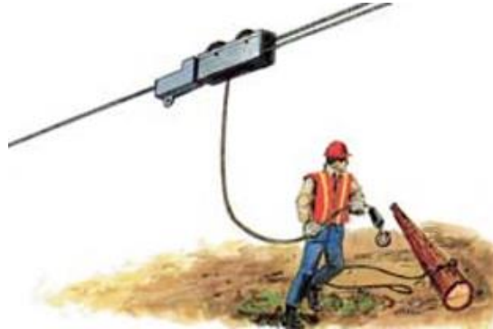
Mechanical stop holding a carriage
