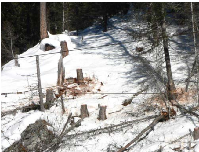
FIGURE 22. One-stump and one tree combined with equalizer block for an anchor in small trees for a small cable-logging system.
