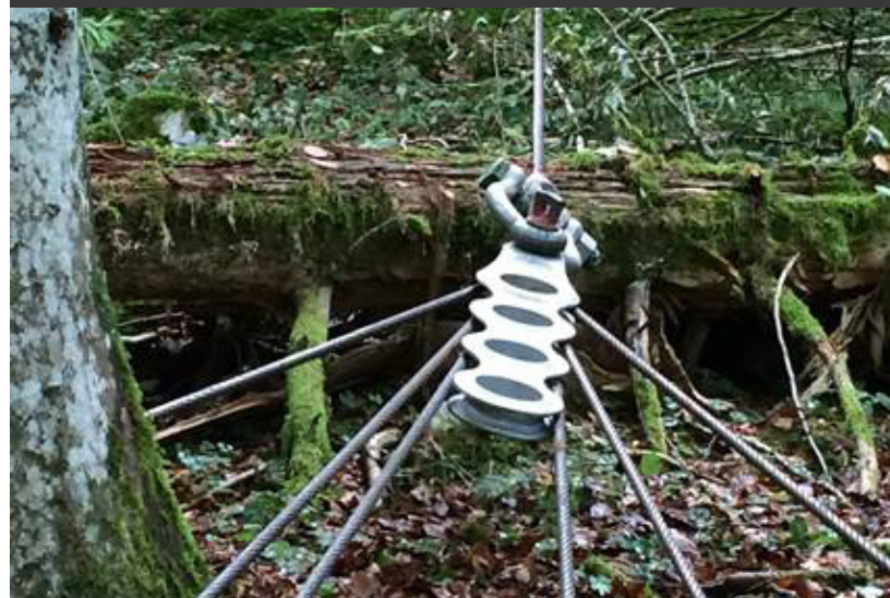
FIGURE 23. Multi-stump/multi-tree anchors used with winch-assist systems.
