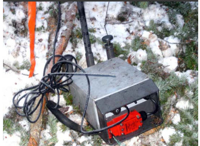
FIGURE 25. Device to detect stump movement.
