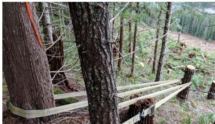
FIGURE 23. Multi-stump/multi-tree anchors used with winch-assist systems.
