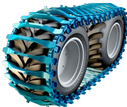
FIGURE 7. Use wheel tracks to prevent wheel spin in slippery conditions
