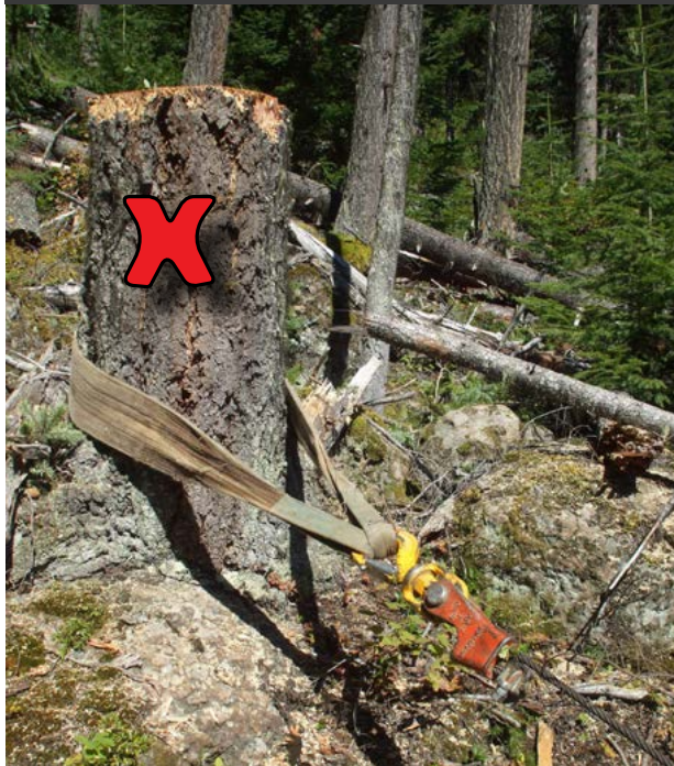
FIGURE 19. Avoid anchor stumps that are perched on rock outcrops.
