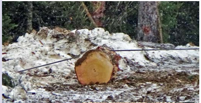
FIGURE 5. Brow log to protect the cable at ground break. Sharp rocks can damage or increase cable wear.
