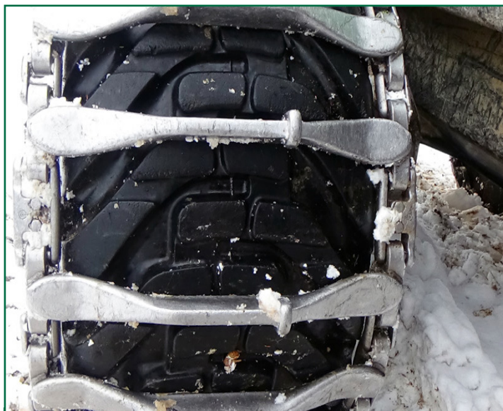
FIGURE 7. Use wheel tracks to prevent wheel spin in slippery conditions
