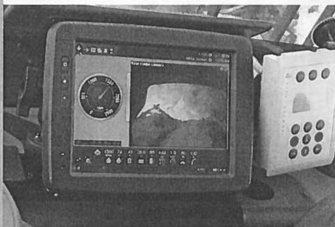
FIGURE 6. A camera is usually mounted at the rear of the forwarder (top) so that the trail behind the machine is always visible from within the cab (bottom).
