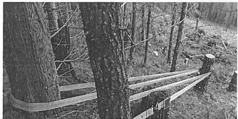
FIGURE 24. Multi-stump/multi-tree anchors used with winch-assist systems.
