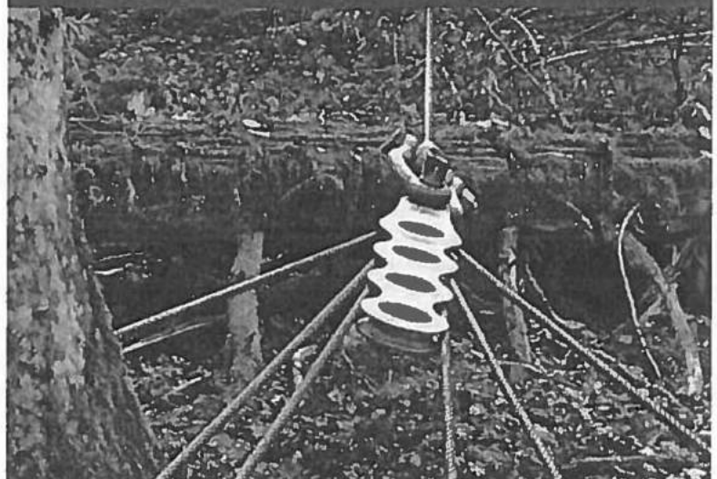
FIGURE 24. Multi-stump/multi-tree anchors used with winch-assist systems.
