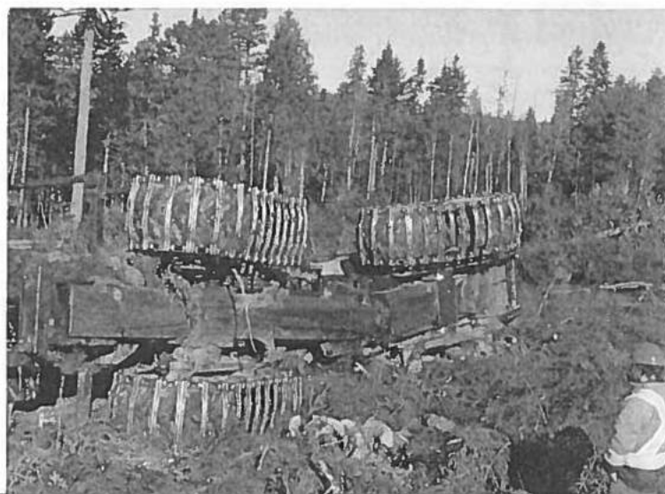
FIGURE 37. Machine that failed to regard the side slope safety recommendation of 5%.
