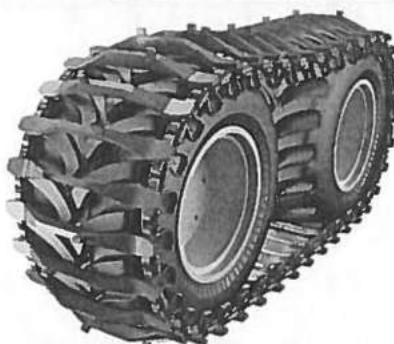
FIGURE 8. Use wheel tracks to prevent wheel spin in slippery conditions.
