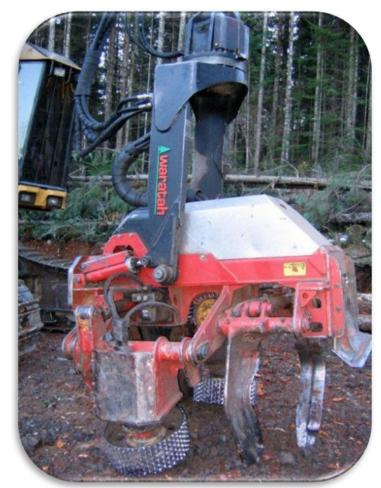
Processing head correctly de-energized for maintenance
