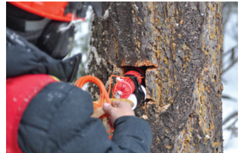
Prepping trees with the right cut (position and size) for the appropriate blasting material to control the blast and fall of the tree as intended, and documenting everything.
