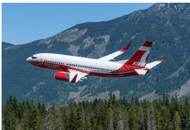
Coulson created the first Fireliner, a converted Boeing 737-300 aircraft, in 2017. Derek Heyes Photo
