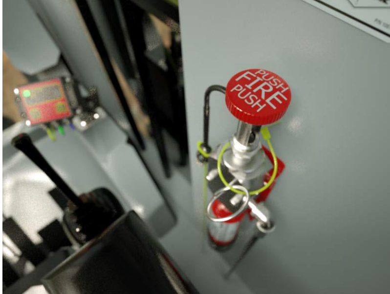
Figure 9. Manual activation device (photo credit Amerex Corp.).
