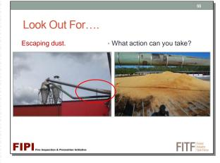
When you observe dust escaping the dust transport ductwork or collection vessel, it means the ductwork in state of disrepair.
