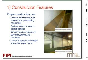
Construction features, such as surface slipperiness, sloping, and sealing, can reduce the accumulation and spread of wood dust.
