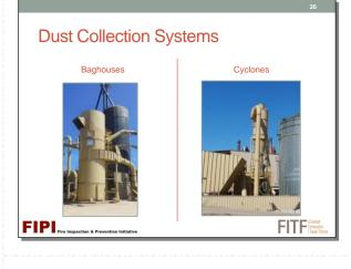
The photo on the right is an example of a cyclone where the dust is separated from the air and collected at the bottom of the cyclone and the clean air is exhausted at the top.
