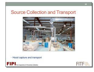
Earlier, we mentioned that the point of capture is the typically the weakest link, primarily because the design of dust capture hoods is not widely understood.
