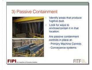
Another type of engineering control is passive containment. Ensuring that passive containment is the right control option is important. Like dust collectors, passive containment creates an environment with the potential to have 4 of 5 explosion pentagon elements present with the ignition source being the only missing element.
