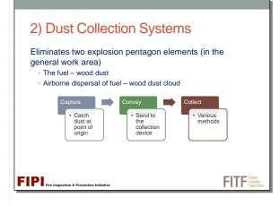
The best mitigation strategy is to capture the dust at the point where it is produce so that it cannot spread and accumulate throughout the general workplace.
