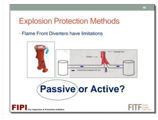
A flame front diverter prevents flames from propagating from one piece of equipment to another through the interconnecting piping.
