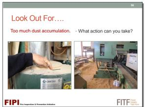
The photo on the right shows a very heavy accumulation of primary dust. The finer dust particles in an accumulation like this, when disturbed, become airborne and settle on flat surfaces away from the machine centre, like for example, as shown in the photo on the left.
