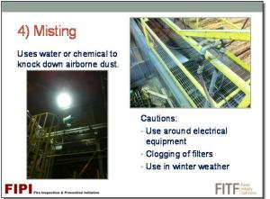
Misting knocks down airborne dust using water or a chemical.
