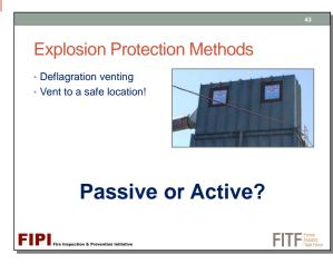
Deflagration Venting is an explosion protection method where a panel or door is provided to relieve the expanding hot gases of a deflagration from a process component or room.
