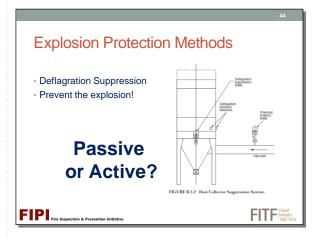
Deflagration Suppression uses a high-speed flameextinguishing system to detect and extinguishes a deflagration before destructive pressures are created.
