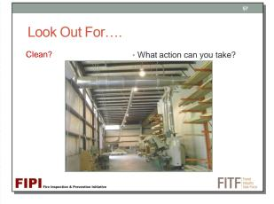
The photo on this slide shows a very clean workplace with the machine centres connected to a dust collection system.
