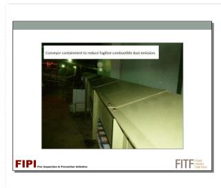
Material conveyance systems can release wood dust into the general work area and elsewhere. This can be reduced by fully or partially enclosing the conveyance system.
