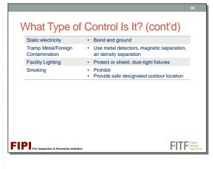
To protect against static electricity, the most common control is to "bond and ground," which is an engineering control.
