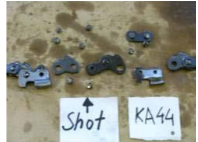
Linkages from a failed chain
