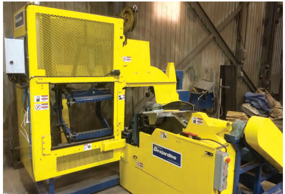
Left and right: The Desjardin Head Saw Guard (yellow) is shown off to the side of the saw (left) and then enclosed around the machinery to support improved safety.
