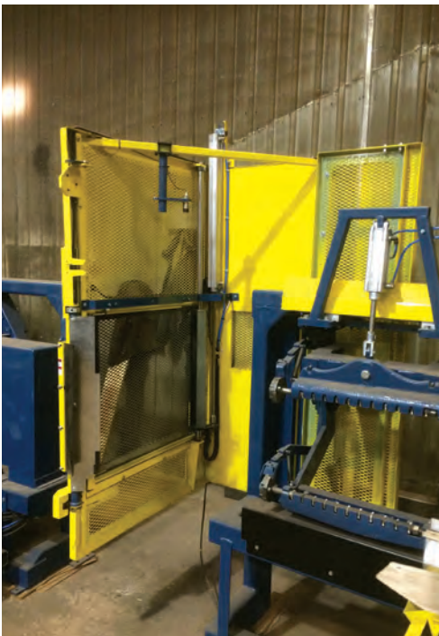
Left and right: The Desjardin Head Saw Guard (yellow) is shown off to the side of the saw (left) and then enclosed around the machinery to support improved safety.
