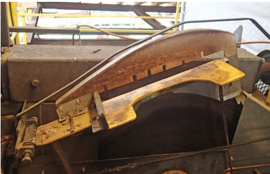
Top: West Coast Solution Head Saw Guard – additional guarding will be put in place for both sides of carriage. Bottom: Trim Saw Guard.
