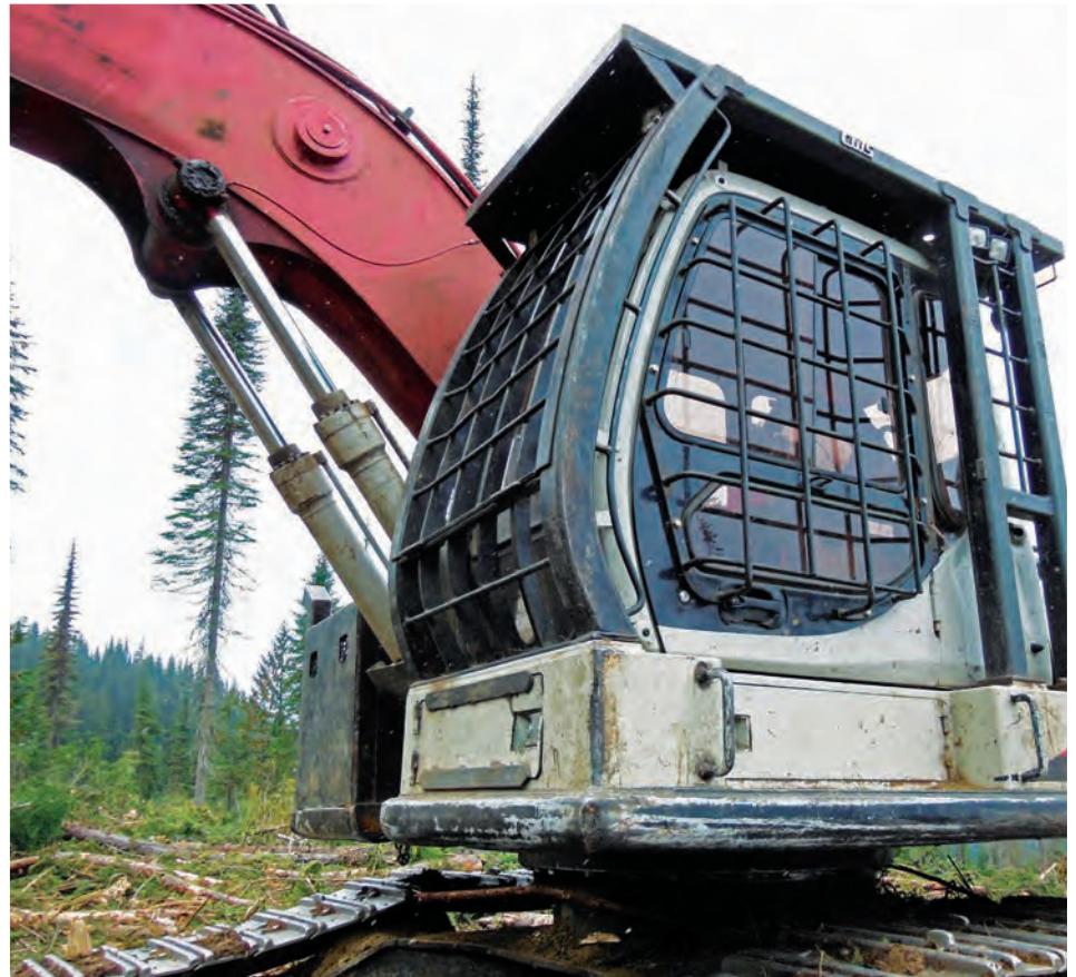
Making sure all mobile equipment has the correct cab guarding and exits for easy escape is a regulatory requirement.
