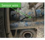
The bend radius should not be less than 10 times the wire diameter. The wire should be routed straight out of connector for a minimum of 8 cm before bending.
