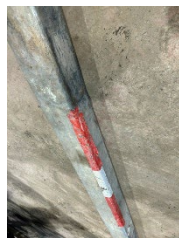
c) Stake bent due to loader interaction
