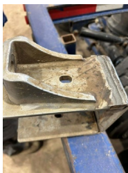
b) Broken bunk securement clamp
