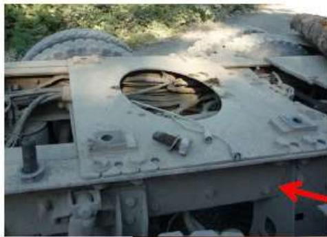
Tractor deck with broken scale pad bolts
